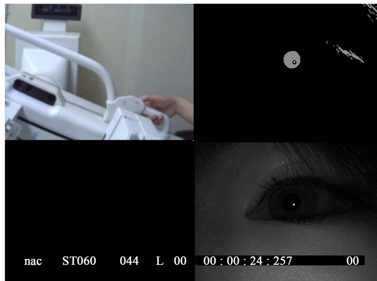
Figure 2. Screenshot captured from video output of the Eye Mark Recorder (upper left: view image, bottom right: eye image, upper right: binary image with pupil region automatically detected from eye image, bottom left: blank).
