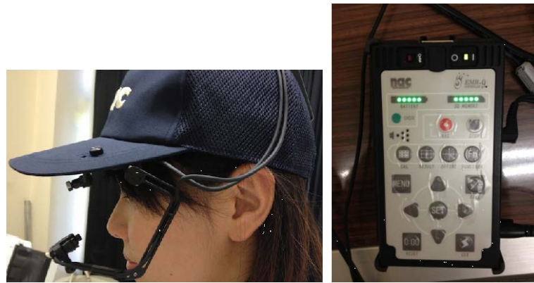
Figure 1. The Eye Mark Recorder used to measure pupil sizes (left: cap-type head unit, right: control unit).
