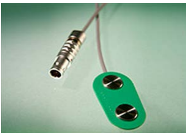
Figure 2. Bipolar surface EMG Electrodes (model SX230, Biometrics Ltd., Gwent, UK) [7].
