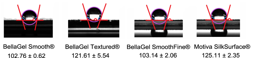
Figure 3. Contact angle analysis of BellaGel SmoothFine® implant. The assessment of contact angle of BellaGel Smooth®, BellaGel Textured®, BellaGel SmoothFine®, and Motiva SilkSurfaces® was carried out using a contact angle meter Phoenix-MT(T) (SEO, Suwon, Gyeonggido, Korea). The experiments were undertaken three times to ensure significance of the tests.
