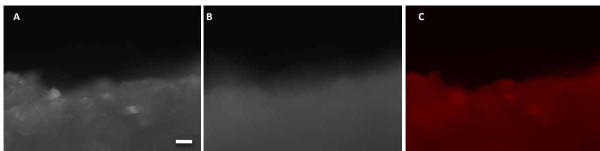
Figure 4. Fluorescent microscope image of fluorescent peptide modified nano-macroporous bioactive glass (A) at the surface, (B) 800 \mu\text{m} into the surface and (C) z-stack image of 10 images between the surface and the upper working depth of the microscope objective of a scaffold modified with 0.01 mole % fluorescent RGD peptide-silane: 1 mole Si. Scale bar = 50 \mu\text{m} .
