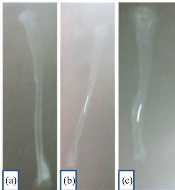
Figure 4. Radiograph for the bone: (a) control; (b) after implantation of \text{TiO}_2/\text{Ti} and (c) after implantation of Ti. The light line in the bone indicates to the plate of implantation.
