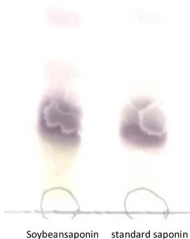
Figure 3. Thin layer chromatography. TLC of soybean saponin after column chromatography and standard saponin.
