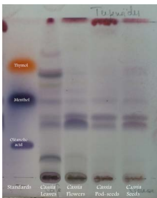
Figure 5: TLC chromatogram of dichloromethane extracts from C. occidentalis with oleanolic acid, menthol, thymol as standards; developed with toluene/ethyl acetate (93:7; v/v) and visualized at visible with sulfuric anisaldehyde reagent. Terpenes are detected as violet spots.
