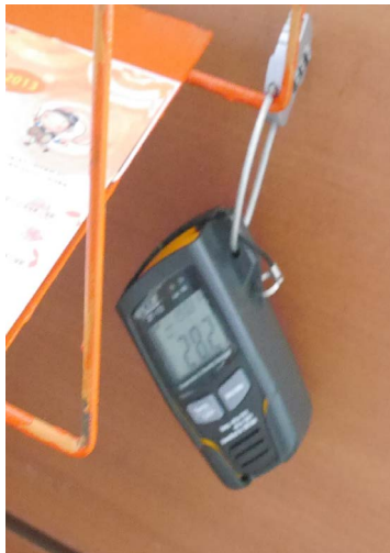
Figure 9. Measurement of indoor temperature and humidity.
