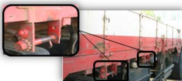
Figure 2. Fixing blocks welded to a truck [6].
