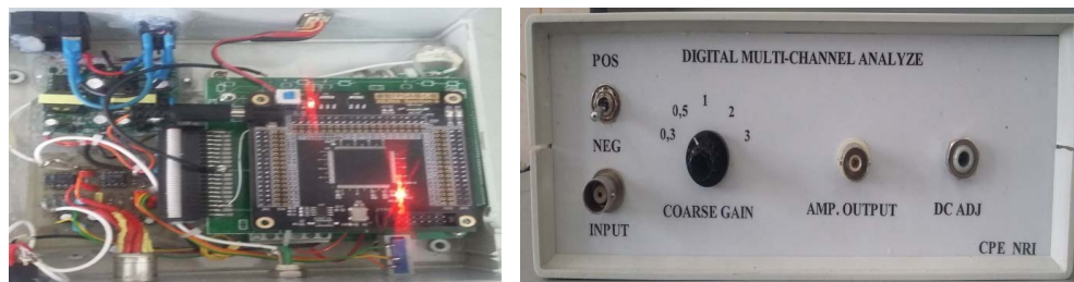
Figure 3. Layout of the DMCA on the left and its front on the right.
