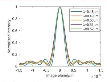
Figure 3. Normalized intensity of the system at the image plane at different wavelengths.
