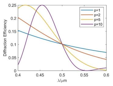
**Figure 2.** Diffraction efficiency varies with wavelength at different p values, the design wavelength is 0.5  $\mu$ m.
