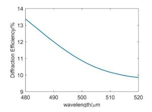
Figure 4. The diffraction efficiency of the scaled down system.
