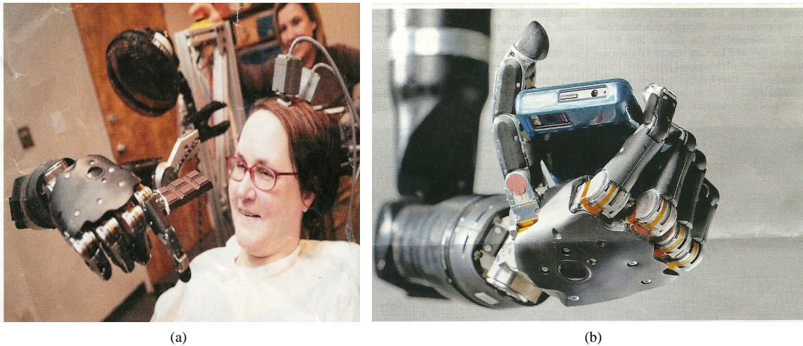
Figure 2. (a) Brain-controlled mechanical arm and hand (Reardon, [42]), (b) “imagine that!” a brain-controlled mechanical hand (Pruszynski and Diedrichsen, [43]).
