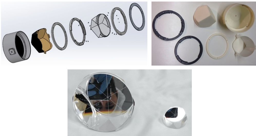
Figure 4. Exploded view of MoonLIGHT (top left). Photos of 3D-printed plastic components of MoonLIGHT (top right). Photo of the MoonLIGHT CCR and of an Apollo CCR (bottom).
