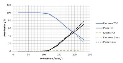
Figure 6. Relative contributions of electrons, muons and pions to the piM1 particle beams.
