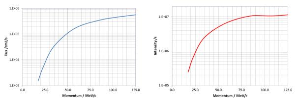
Figure 7. Maximum values of the electron flux and intensity for proton beam intensity of 2.1 mA.
