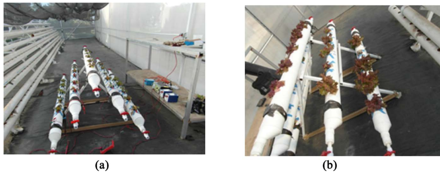
Figure 4. Experiment 2. System to apply the different intensities of DC to galvanostatic regime (a). Inferior container (R-5), it fed with the smallest intensity of direct current and it contains the plants of more growth (b).
