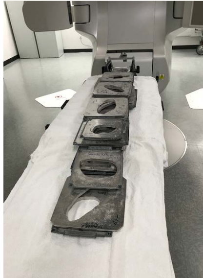
Figure 3. Weights (used cerrobend block) weighing 200 pounds were placed on the couch to imitate the patient weight.
