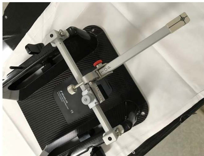
Figure 4. The phantom, adjusting device, and supporting base.
