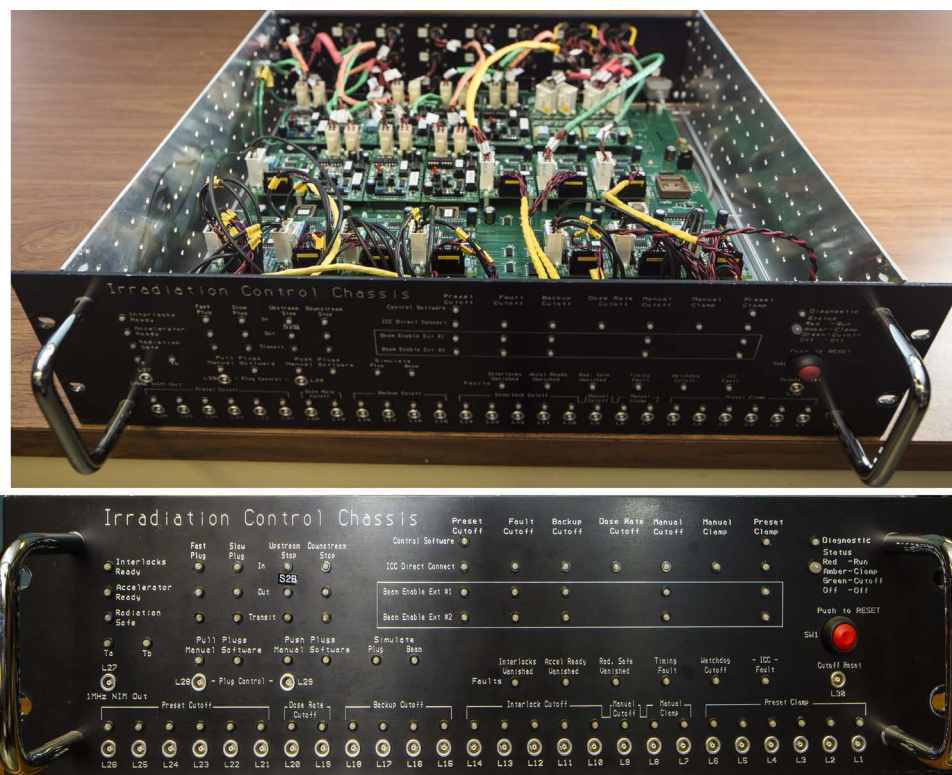
Figure 7. Shows the irradiation control chassis (both front and top views).
