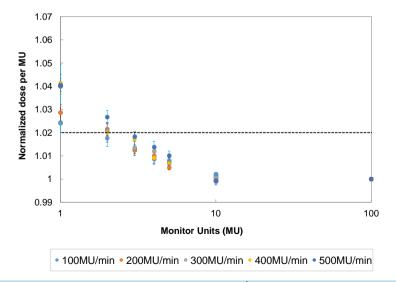
Figure 2. Relative delivered dose per MU in a  $(10 \times 10)$  cm<sup>2</sup> field versus the MU setting. Results are plotted for several dose rates. The error bars represent 1 standard deviation based on five measurements. Dashed lines represent the 2% dose variation.
