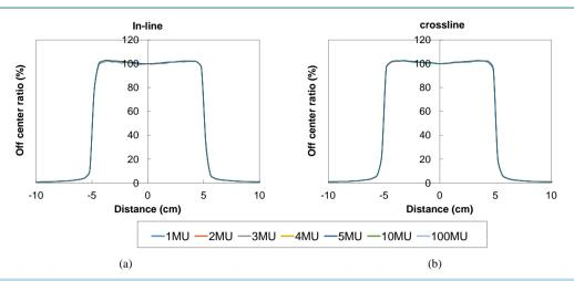
**Figure 3.** Dose profiles of the (a) in-line and (b) crossline at various MU settings under a dose rate of 500 MU/min. Beam profiles were normalized at the central axis (CAX).
