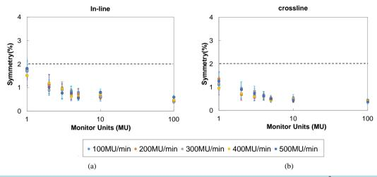
Figure 4. Calculated symmetries of the (a) in-line and (b) crossline profiles in a  $(10 \times 10)$  cm<sup>2</sup> field versus the MU setting. Results are plotted for several dose rates. The error bars represent 1 standard deviation based on five measurements. Dashed lines represent the 2% symmetry variation.
