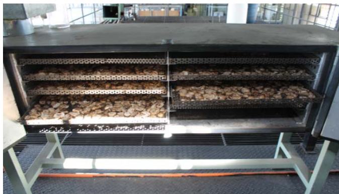
Figure 3. Drying chamber with mushrooms.
