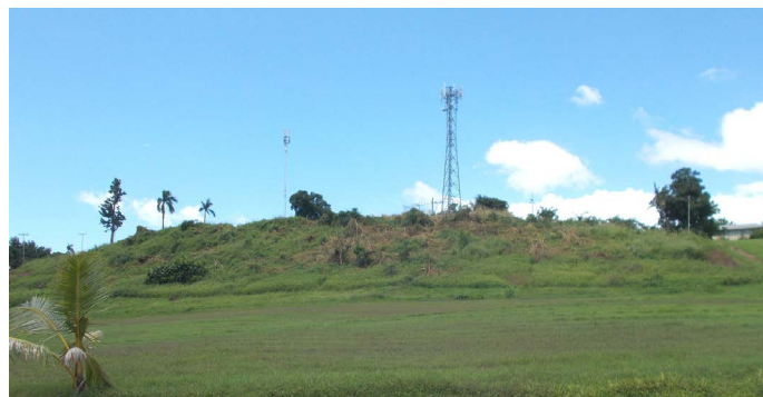
Figure 5. Location of the Lautoka GPS station on a bedrock-hill at an elevation of +89 m. It seems to record a weak crustal subsidence. The tide-gauge station in the harbour rests on soft marine sediments, and is therefore likely to record an additional site-specific loading subsidence due to compaction of the underlying deposits.
