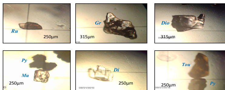
Figure 7. Mineralogy of coarse fractions in polarized light (PL) of analyzed clayey materials of pK27 pyrite deposit. Ru: rutile; Gr: grenat; Dio: diopside; Mu: muscovite; Py: pyrite; Di: kyanite; Tou: tourmaline.
