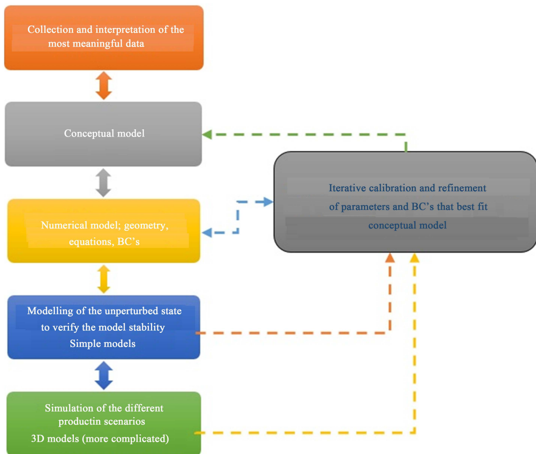
Figure 1. Conceptual scheme for the elaboration of a numerical model of a geothermal reservoir.
