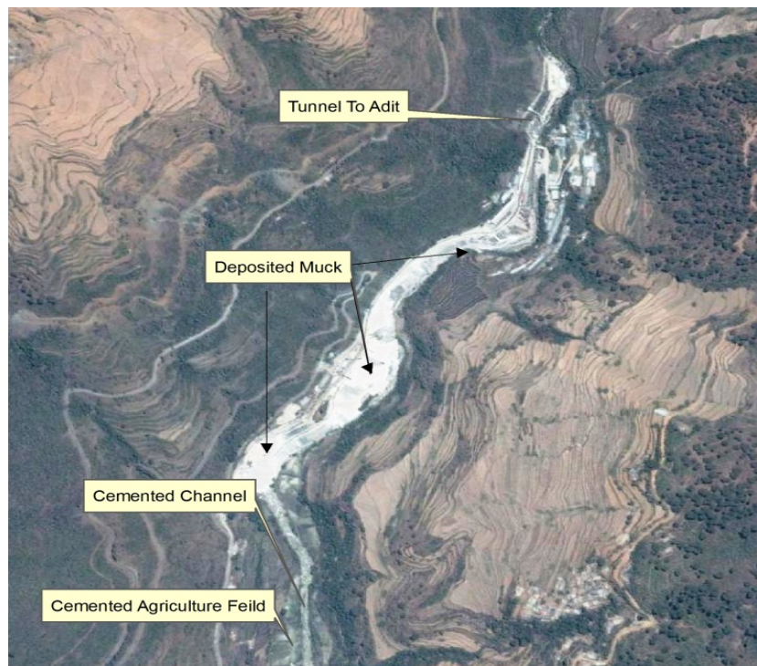
Figure 3. Google Earth® image showing the deposited debris and waste cement along the Dhanari Gad at DhanariAdit.
