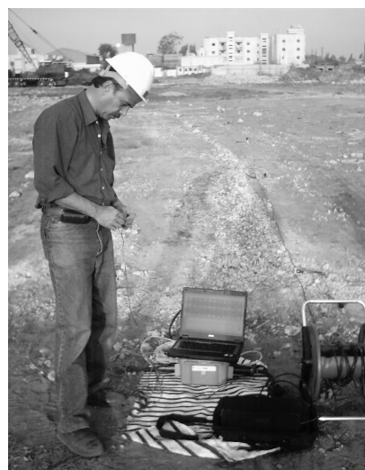
Figure 2. A pictures showing data acquisition for ReMi test using ES-3000 12 channels Geometrics seismograph.
