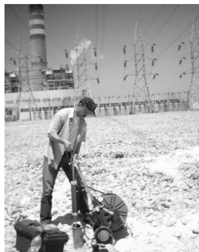
Figure 3. Ballard borehole seismic source S-wave enhanced.
