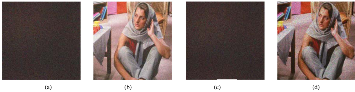
Figure 5. Test of noise attack: (a) encoded image having Gaussian noise with variance 0.1; (b) corresponding decrypted image with all correct keys (c) encoded image having speckle noise with variance 0.1; (d) corresponding retrieved image with all right keys.
