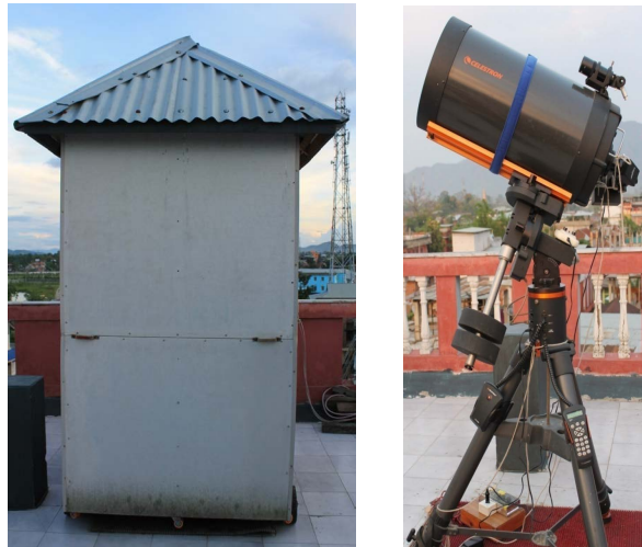
Figure 2. Self-built hut-type observatory (left) and the in-housed Celestron 14" telescope (right).
