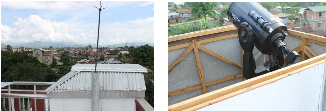
Figure 3. Self-built bullet-type observatory (left) and the in-housed Meade 12" telescope (right).
