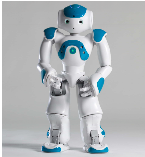
Figure 1. NAO humanoid robot used in this research. The robot is equipped with camera sensors, microphones, speakers and distance sensors [10].
