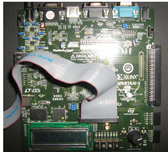
Figure 23. FPGA card with LCD and controlling keys.
