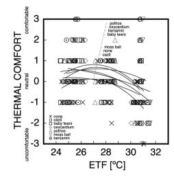
Figure 6. Relation between ETF and thermal comfort.
