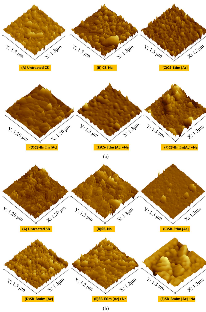
Figure S1. (a) AFM images of Native, IL, NaOH and IL+NaOH pretreated corn stover; (b) AFM images of Native, IL, NaOH and IL+NaOH pretreated sugarcane bagasse.
