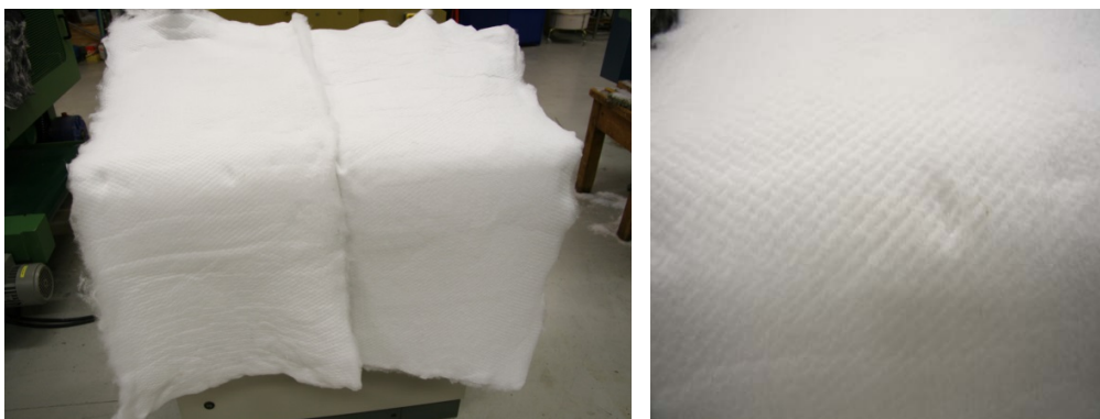
Figure 6. Carded and needled Lyocell mats.
