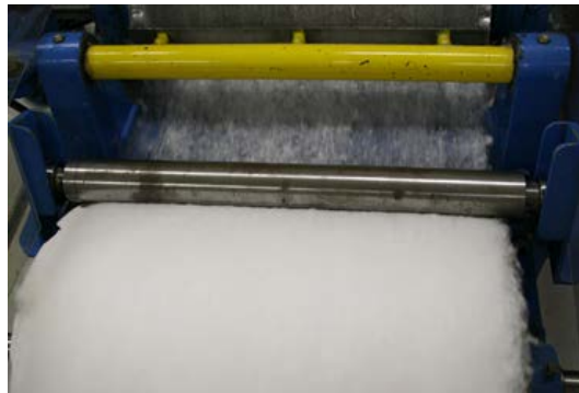
Figure 4. Outlet of the carding machine.
