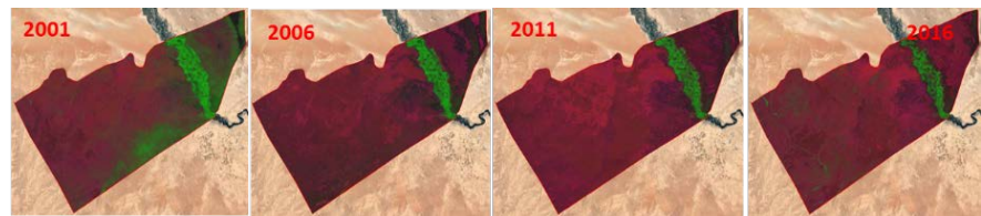
Figure 4. Performance of biophysical image composite (BIC) for the detection and visualization of changes in barren lands from 2001 to 2016 in Abu Kamal, DayrAzZawr, Syria. A large vegetative areas (green pixels) present in 2001 lost in 2006 and 2011, and barren lands (red pixels) increased substantially. Some regrowth of vegetative areas (green pixels) was noticed in 2016. The BIC images were overlaid over the Google Map images.
