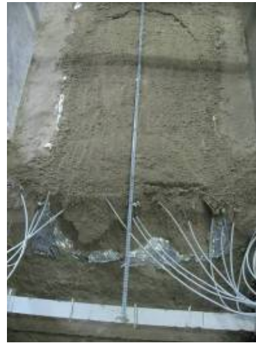
Figure 4. Critical state of landslide body with thickness of 10 cm.
