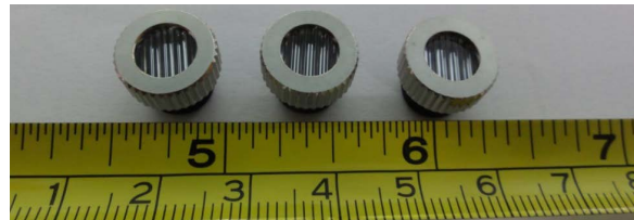
Figure 2. Laser dot to laser line optical converters, 60, 90, and 12 degrees from left to right. Multiple rod lenses are aligned so they are reminiscent of Fresnel lens. Referred as pseudo-Fresnel lens in this research.
