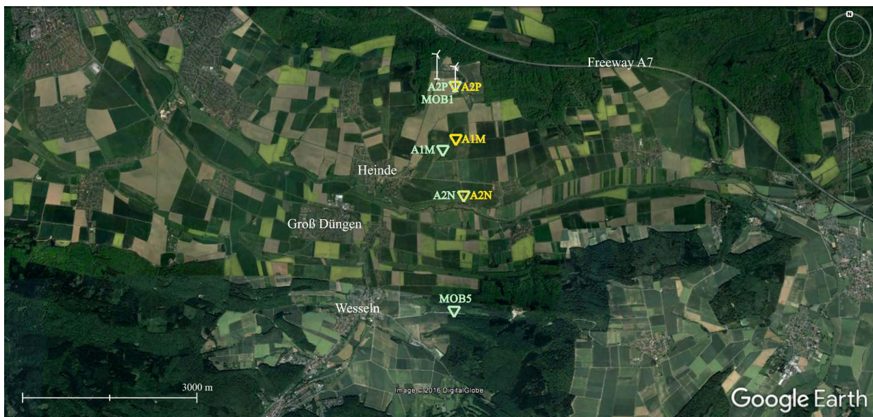
Figure 4. Measurement campaigns at WP Heinde, near 45 km to the south of Hannover. During the first campaign, the stations were located at 10, 1000 and 2000 m from the wind turbine to the south (yellow triangles). The second campaign recorded with four stations with distances of 10 m, 1.2, 2 and 4 km (green triangles). Station A1M of the second campaign recorded during 1 week in order to analyze the noise temporal variation.
