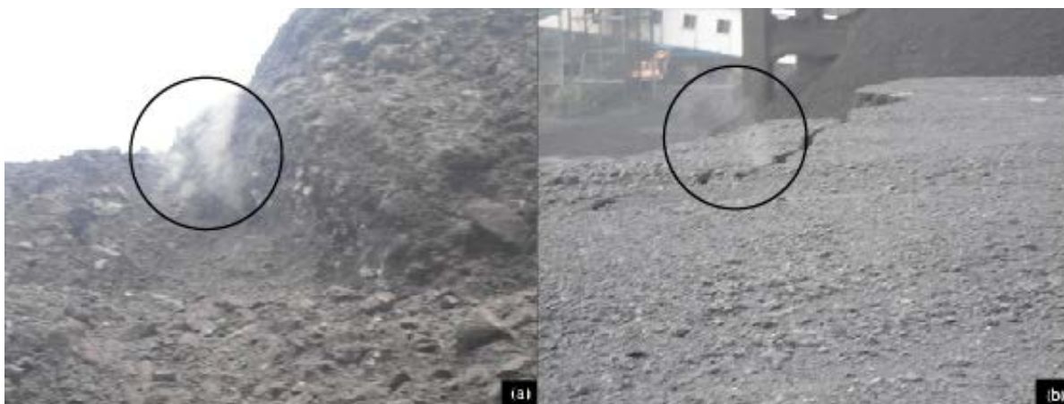
Figure 2. Smoke produced by the action of self-heating of coal in Barapukuria coal stockpiles, (a) smoke found in the pick of the coal stockpile, (b) smoke produced through crack that occur during loading coal.
