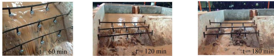
Figure 2. The failure characteristics of the earthen embankment; overtopping case (at Q = 16.84 l/s).
