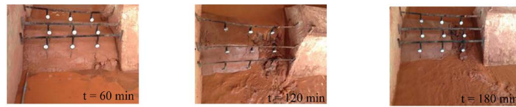
Figure 5. The failure characteristics of the earthen embankment; beneath structure case (at Q = 16.84 l/s).
