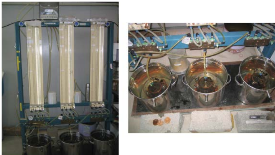
Figure 8. Device of falling head permeability test.
