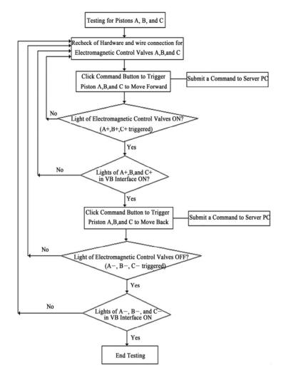
Figure 7. A system testing diagram for a remote-controlled three-axis robotic arm.
