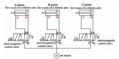
Figure 3. The diagram of the pistons with respect to three electromagnetic control valves.
