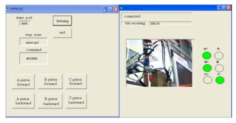
Figure 5. The manual movement of the robot's arm on the VB dialogue (pc sever).
