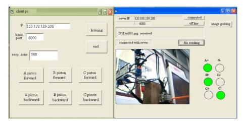
Figure 6. The manual movement of the robot's arm on the VB dialogue (pc client).
