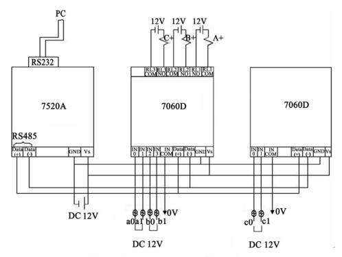
Figure 4. The wire connections of the modulus.
