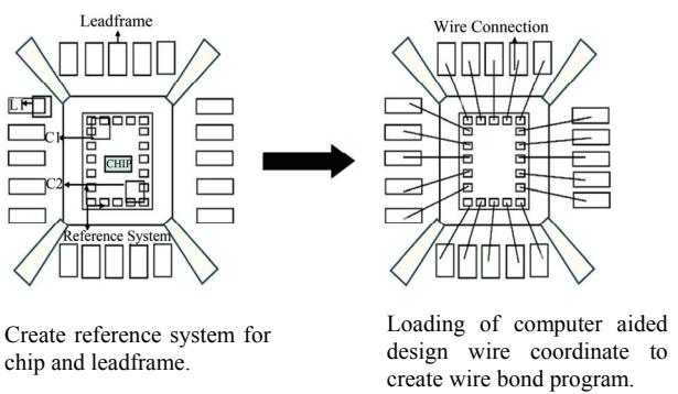
**Figure 2.** OLP allows all wires to be created in bonding program simultaneously.
