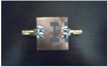
Figure 2. Fabricated DGS unit at resonance frequency 5GHz.
