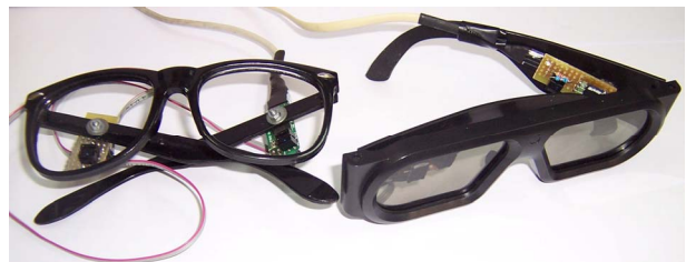
Figure 3. Human-machine interface of biomechanical signals for the detection of voluntary winks.
