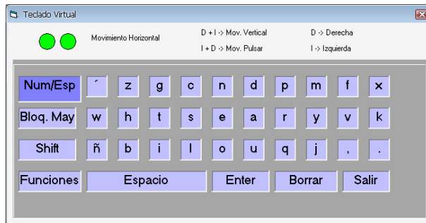
Figure 6. Virtual keyboard aspect with the letters ordered according to their Spanish utilisation frequency.
