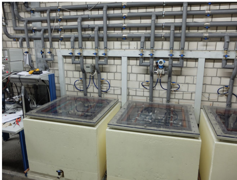
Figure 1. Heat storage shelter of polypropylene with content of 400 litres.
