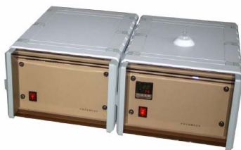
Figure 1. NMR mud logging unit.
