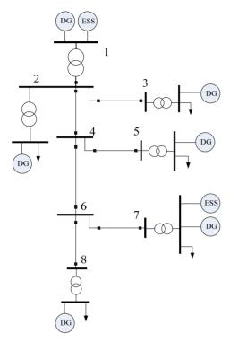
Figure 1. AC topology of a stand-alone microgrid system.
