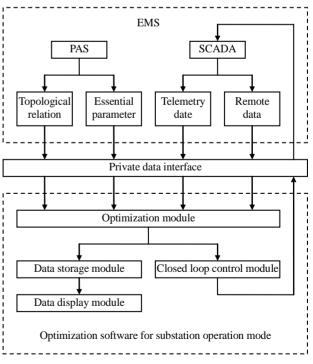
Figure 1. Framework of optimization software for substation operation mode.
