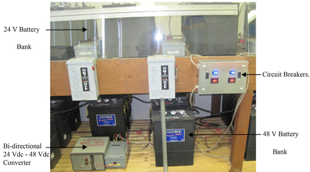
Figure 13. Actual operation of the bi-directional DC-DC converter.
