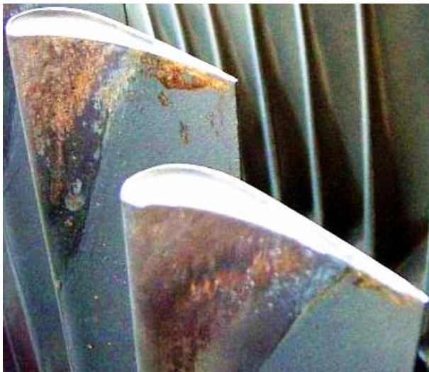
Figure 4. Damage by erosion in the working blades of the last stage in a steam turbine of 300 MW (Picture of Rueda4, 2006).
