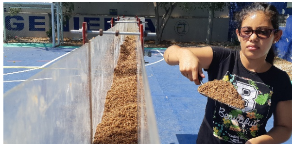
Photo 3. A student introducing coarse sand from the Suchiapa River in the hydraulic channel.
