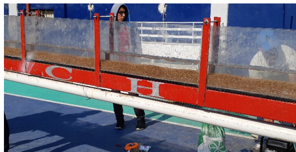
Photo 4. Water flow of 2 l/s and v = 0.5 m/s during 4 h.
