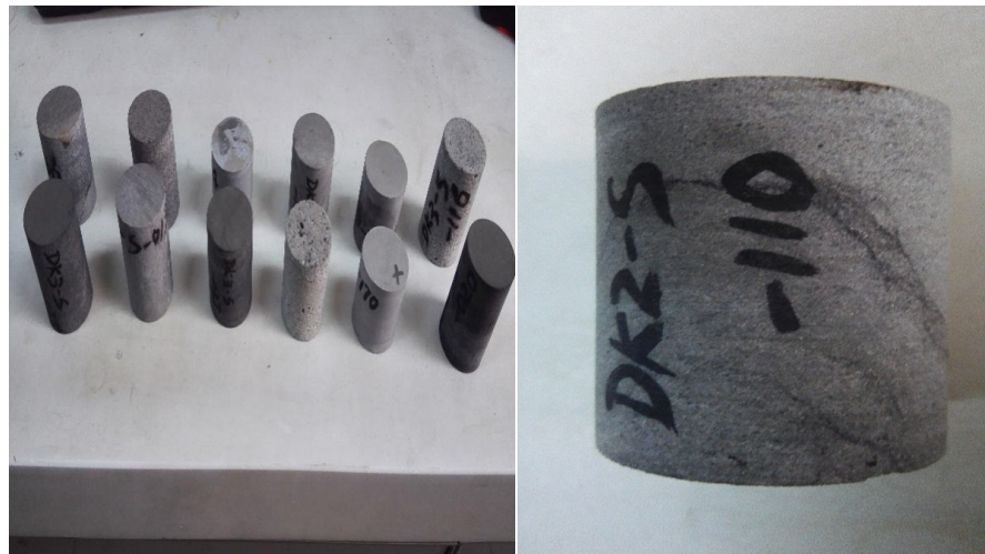
Figure 1. Photos of samples (The left is the samples. The right shows the fractures). (a) Samples; (b) Fractures at the surface.
